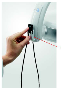
Sopix/Sopix 2 Inside sensor holder properly installed
